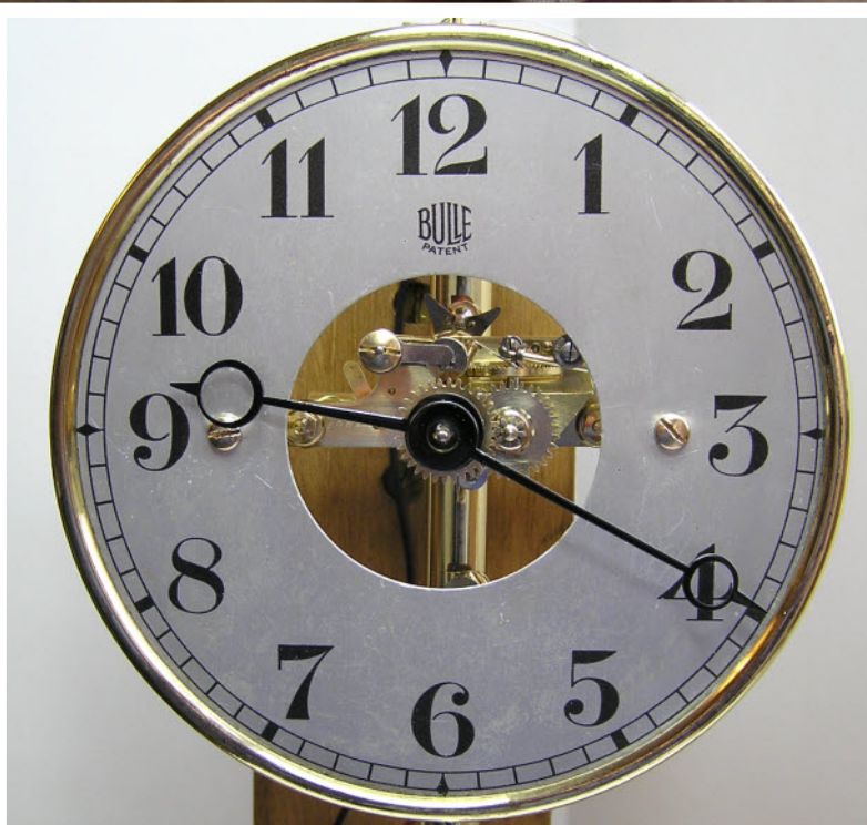
The dial after cleaning and polishing the surround.
