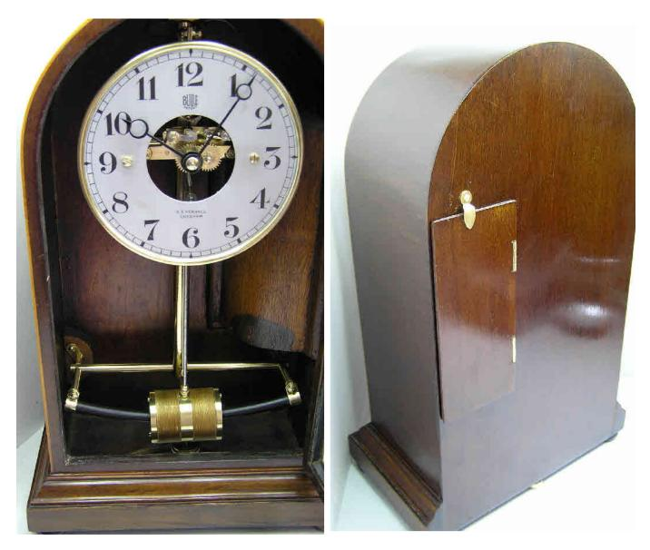
The clock replaced in the case ready for fixing on the door. The back of the clock is shown with the battery door in place. The whole case was in good condition and only needed a good buffing with beeswax polish.
