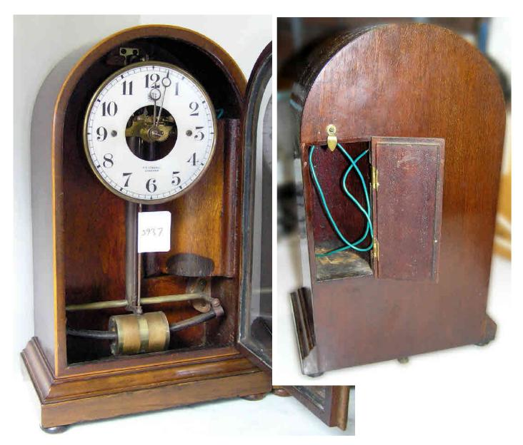
The restoration will be of serial number 5937. The clock looks to be complete with little damage if any. It is obvious that the wiring has been changed at some time though. The battery compartment looks generally clean and free from any acid damage.
