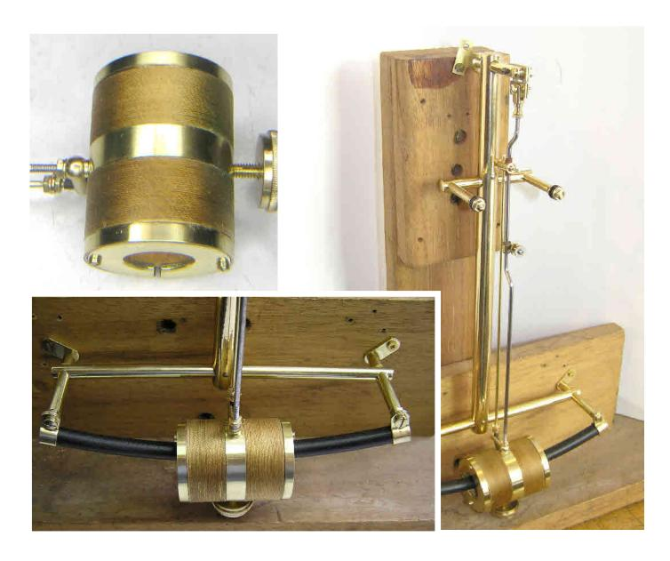
This sequence of photos show the pendulum bob that has been cleaned whilst still keeping the original cord intact. This takes a lot longer but can be done if the cord is in a good condition. The magnet has be re-magnetised, cleaned and "Grate Blacked". The frame is then shown on a test stand with the pendulum assembly attached for testing lengths and clearances.
