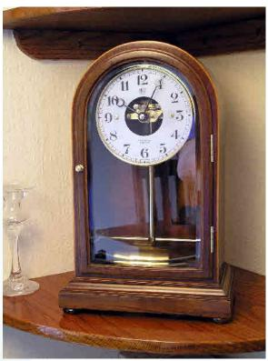
The case has had all the brass work removed, cleaned and polished. The glass is thick and bevelled and runs the whole length of the case to show off the movement to great effect.
