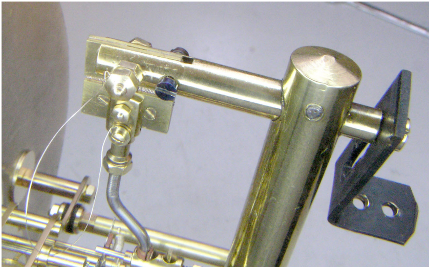
The pendulum assembled with the frame using the new parts. Note the two new blue steel crews that grip and position the top of the silk suspension.. The photo at right shows the whole movement, pendulum and frame with the case brackets ready for insertion into the case.
