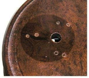
The photos left and above shows the three extra holes (circled) in the bakelite base. The column is now offset with only a third of the hole up the column visible from underneath. It is only by luck that the holes are not visible from the top when the column is in position. The wide base of the chromium plated column extends over them as can be seen from the dark area in the photo left. I have no idea why it was done.
