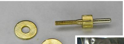
The new parts for the contact pin assembly ready to be attached. The body of the assembly has been threaded to accept the new silver contact pin.
