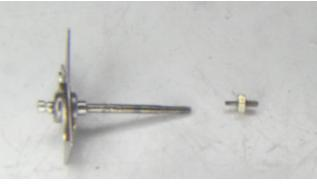
There is nothing wrong in this type of repair other than the wrong adhesive used. So I will clean it and reattach with Loctite 603.
