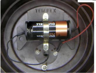
The underside of the bakelite with the new battery holder in place. I used the existing screw holes for this and made a small frame from some scrap brass to support the battery.
