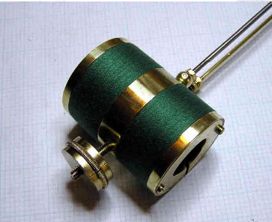
Some close ups of the pendulum and the reassembly Isochron attachment. This attachment needs to be completely isolated from the pendulum and has a small Emery Cloth type insulator between it and the pendulum rod.
