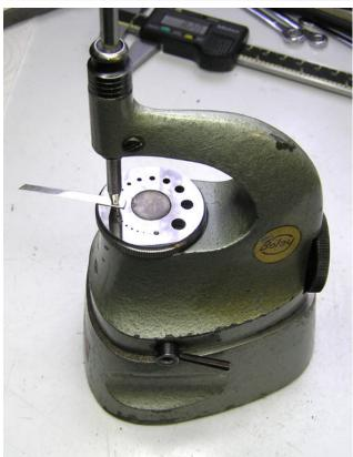
The first stages in making the replacement fork contacts. I use hard fibre washers which are then roughly cut to shape and thinned before fitting. Once in place I can finely shape with a disc cutter and needle files. The edge is then polished smooth.
