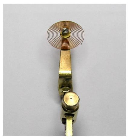
As I first suspected on seeing this clock very little was damaged or missing. So apart from the Balance contact spring and the Fork contacts the rest of the clock was in good order and just needed a strip and clean. These photos show the new spring and the finished pendulum about to be re-united with the dial plate.
