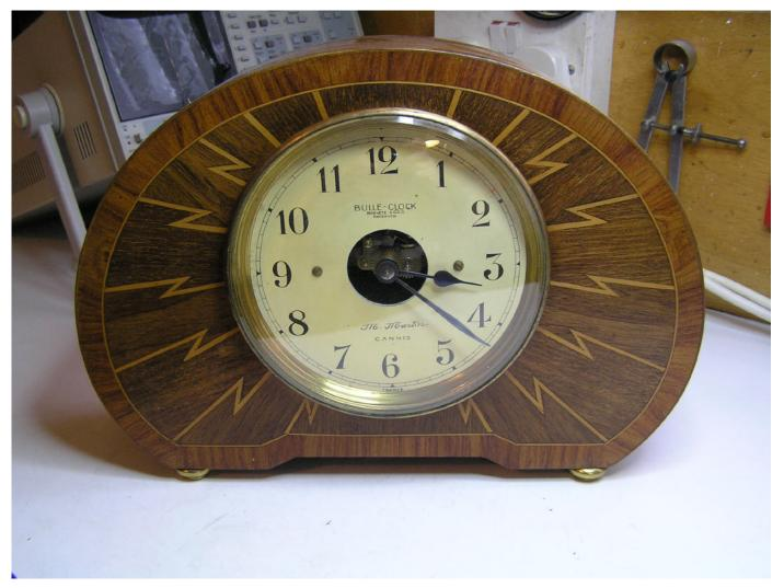
This clock is a model XA in a wooden "Lightening" case. The movement will be shown undergoing restoration by kind permission of the owner. As can be seen from this photo the casework and brass fittings are all in very good condition and other than a good wax polish will no require any remedial work. The brass still retains most of its original gilding and any heavy polishing will remove it. The glass will be removed and cleaned.
