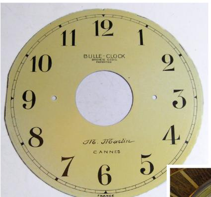
The dial is generally in good condition and suffered only from a grimy surface. This was easy to remove with just a little warm soapy water. It is difficult to tell whether the yellowing is caused by smoke or whether it was originally this colour.
