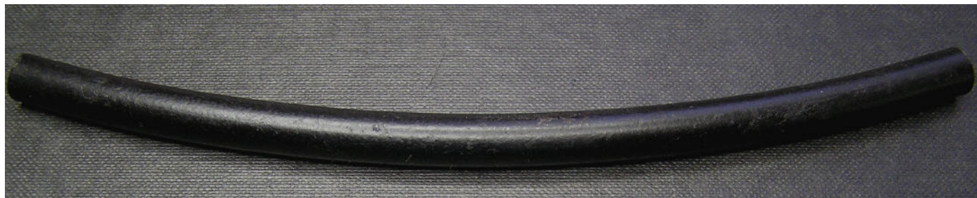
The bar magnet after regenerating and buffing with Grate Black.
