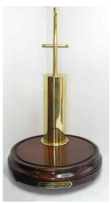
The column has been cleaned in the usual way with Horolene, White Vinegar and finally Bicarbonate of Soda to neutralise the acid.
