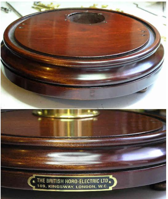
The base after cleaning and French Polishing. There are about 8 coats on this base which have then been cut back to leave a nice lustre. Note in the top photo the indentations left by the brass nameplate which was missing when received.
