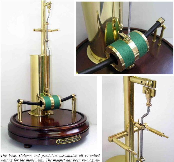
The base, Column and pendulum assemblies all re-united waiting for the movement. The magnet has been re-magnetised for the normal 3 pole configuration and reads a good 19cm on the magnetometer.
