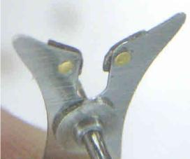
The fork contacts are well worn and will be replaced.
