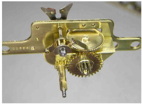
The photos above show the replacement fork arbour ready for installation. Note the small amount of overlap needed on the Fibre contact. This must exactly follow the line of the steel fork leaving ample room for the silver contact pin to freely engage in the fork cheeks.
