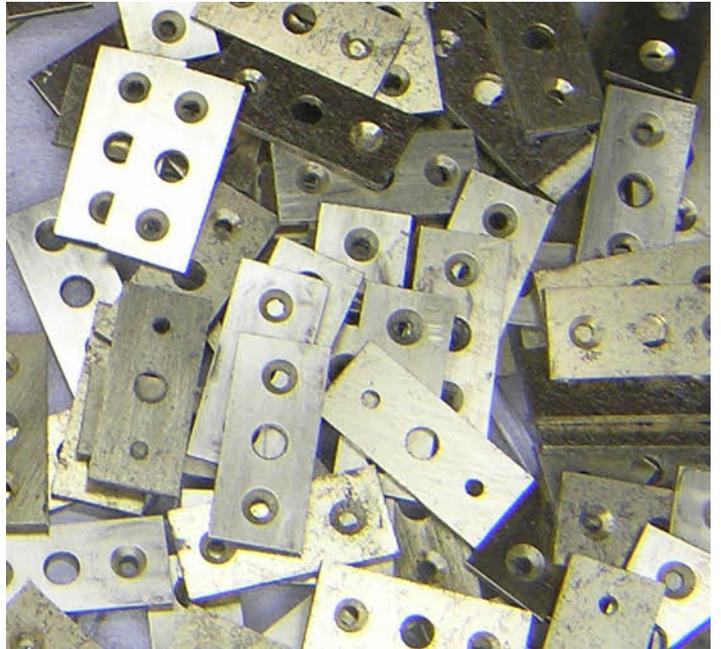
*The top and bottom plates fresh from machining. The first part is the base which has a slot to carry the lead strip that retains the ribbon. The screw holes are threaded for 2mm. The top plates are countersunk for the 2mm screws and do not have a slot.*
